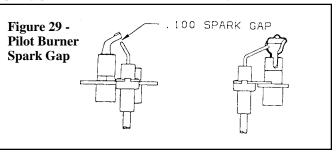
In the event the pilot flame is short and/or yellow, check the pilot orifice for blockage caused by lint or dust accumulation.
